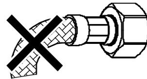
Both ends of the hose must have a minimum 50mm straight section before any bend.
